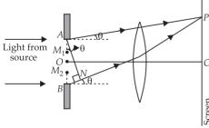
Consider a parallel beam of monochromatic light is incident normally on a single slit AB of width a as shown in the figure. According to Huygens principle every point of slit acts as a source of secondary wavelets spreading in all directions. The mid point of the slit is O.
